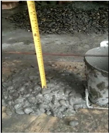
Gambar 3. Pengambilan Nilai Slump Campuran Beton
