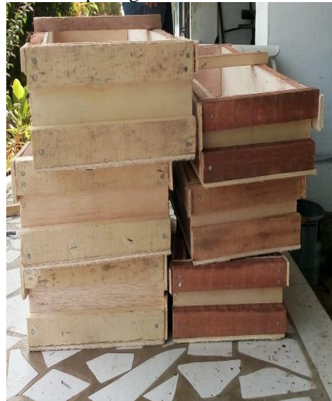
Gambar 1. Bekisting beton benda uji
