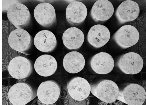
Gambar 1. Material Benda Uji Beton
