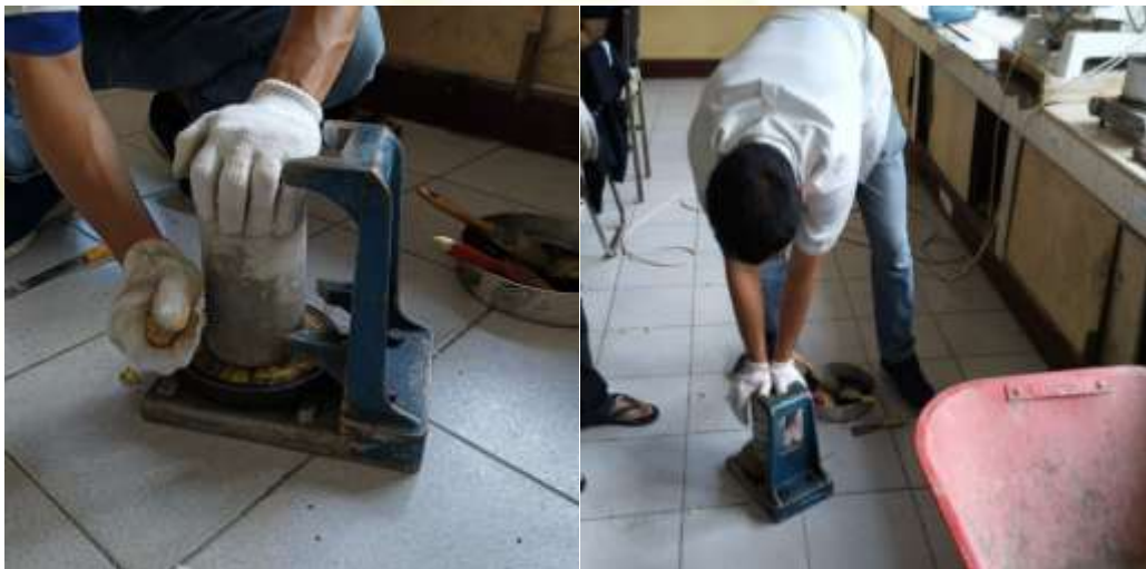
Capping beton silinder
