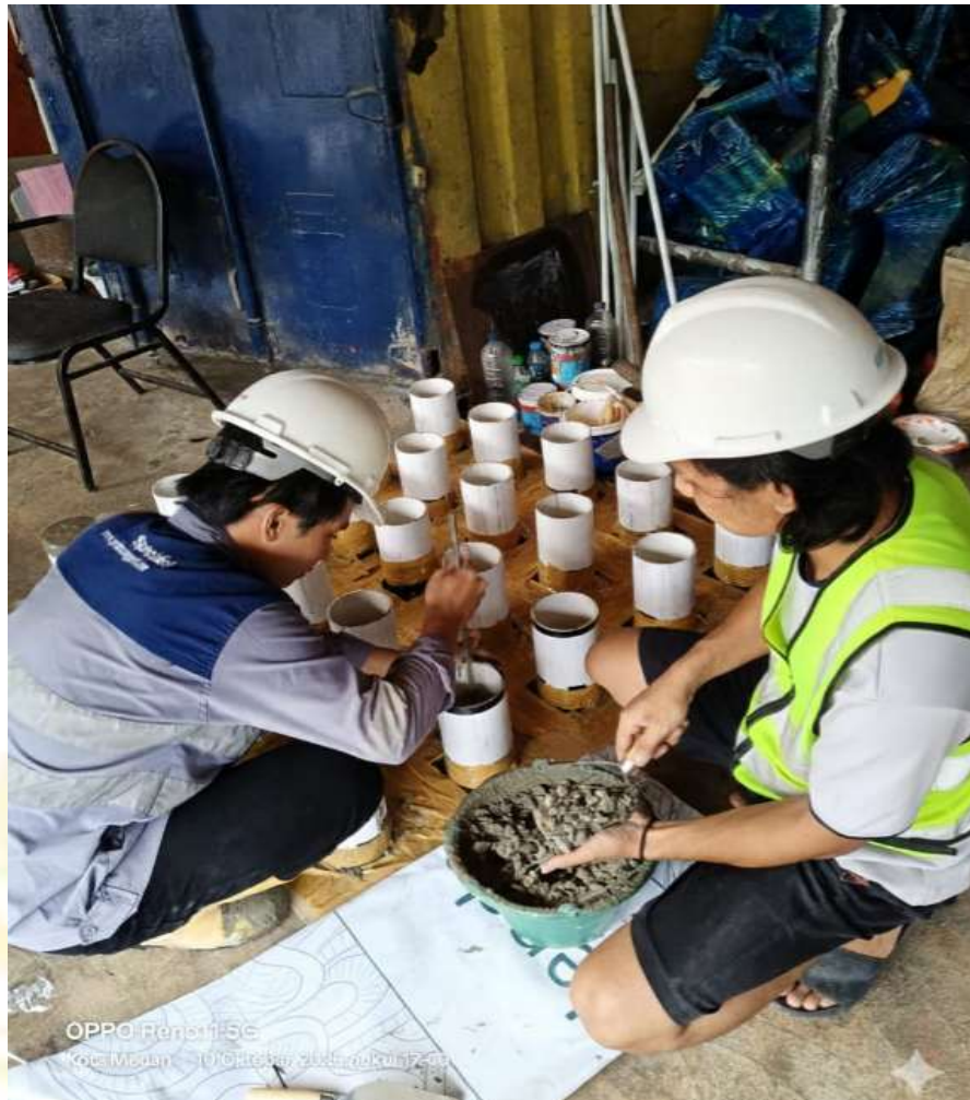
Pencoran beton silinder
