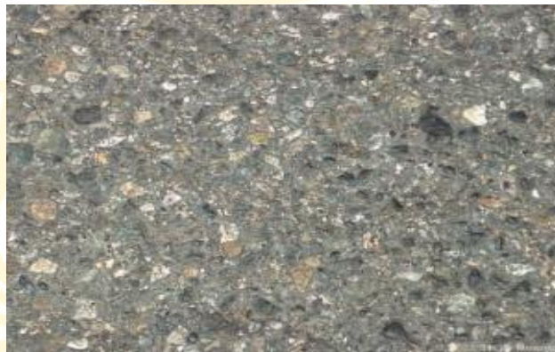
Gambar 2.21 Pengausan ( Polishing ) Sumber: https://www.asphaltwa.com/polished-aggregate/
